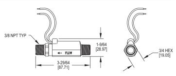
The Series P8 High Pressure Brass Flow Switch is ideal for high in-line pressures. Set points range from 0.25 to 2.0 GPM for liquid flow.
