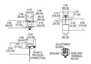
The **Model AAFS Adjustable Air Flow Switch** is capable of detecting a wide range of air velocities with minimal user calibration. The adjustable screw changes the set point at which the SPDT snap switch engages. Quality features include a stainless steel vane, galvanized steel base, and ABS enclosure. The unit is field adjustable from 200 to 1800 FPM (1 to 9.2 m/s).
