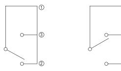
Switch position when air flow is present: continuity between terminal 1 and 2 Switch position when no-air flow is present: continuity between terminal 1 and 3
