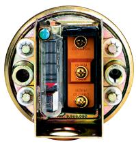
**Note** set point adjustment indicator window. For quick adjustment of set point before/after installation, turn adjustment screw until red bar is at desired set point. To adjust for low gas pressure interlock service, refer to chart (other side).
