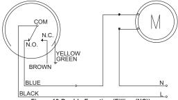
Figure 10-Double Function (Filling (NC)) CFS2-DGXXX-XX
