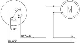
Figure 5-Double Function (Emptying (NO)) CFS2-DNXXX-XX
