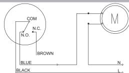
Figure 6-Double Function (Filling (NC)) CFS2-DNXXX-XX
