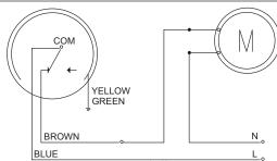
Figure 8-Filling (NC) Function CFS2-CGXXX-XX
