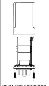
Figure 1: Remove cover to access program switches
