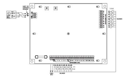
Figure 2-1 Wiring Connections DCT622, DCT632
