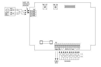
Figure 2-2 Wiring Connections DCT604, DCT606, DCT610
