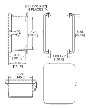
Weatherproof Enclosure Option DCT604, DCT606, DCT610
