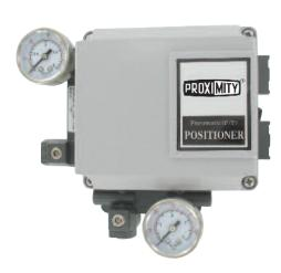
The Series 165NL PRECISOR® Pneumatic Positioner, is used for pneumatic valve actuators by means of pneumatic controller or control systems with an output signal of 3 to 15 psi or split ranges.
